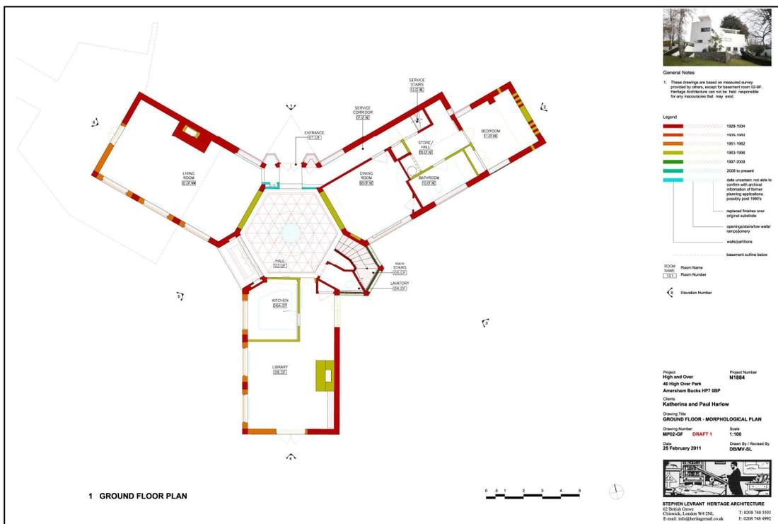
Fig. 5. Morphological drawing reflecting different periods of construction of architectural elements. (Drawing by/courtesy of SLHA)
