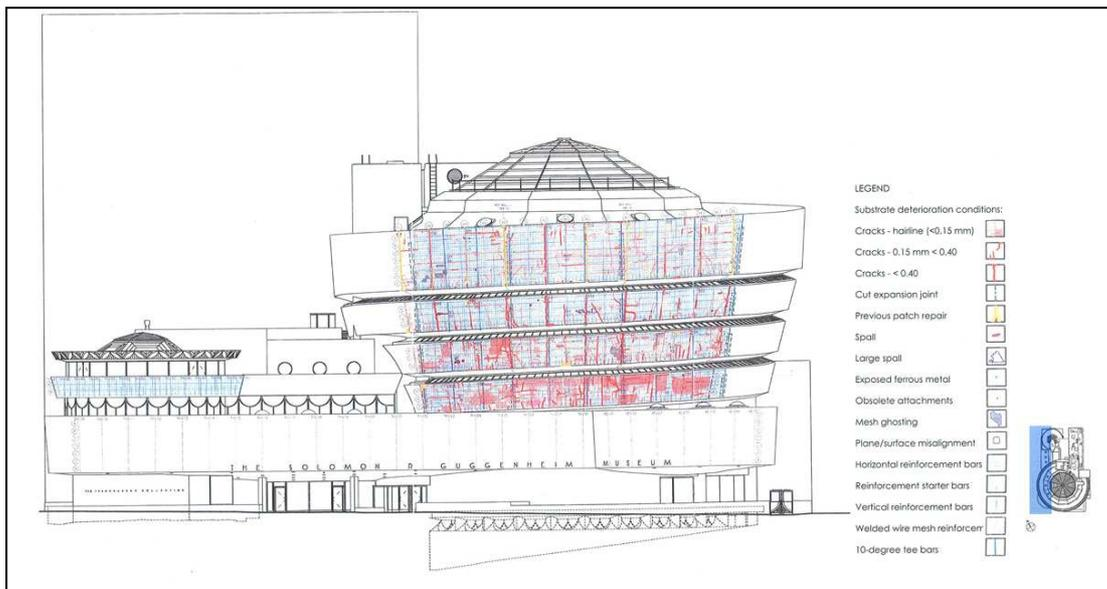
Fig. 4. Overlay drawing showing the correlation between pathologies and the steel reinforcement layout. (Drawing by WASA/Studio A with permission of the Solomon R. Guggenheim Foundation.)
