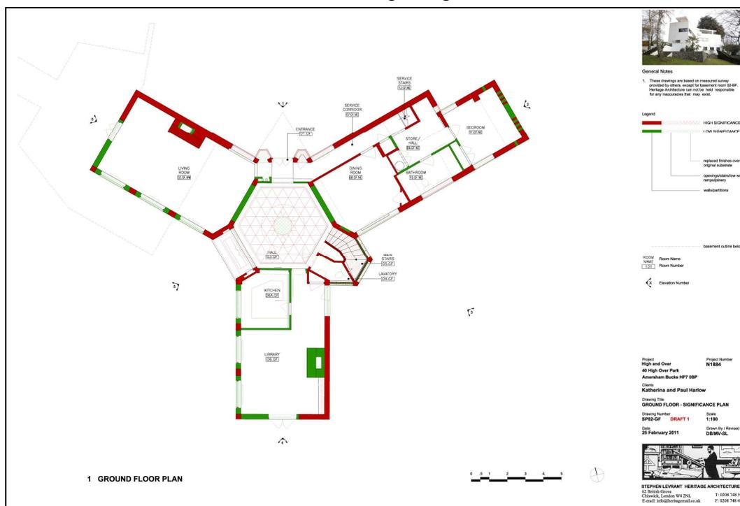
Fig. 6. Significance drawing. Red indicates original construction. Green refers to later, low significance alterations. (Drawing by/courtesy of SLHA)
